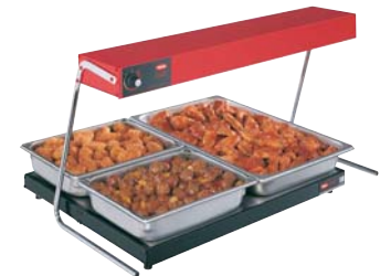
GRA-36 over GRS-30 Glo-Ray Infrared Foodwarmer with optional Designer color and infinite switch and accessory C-leg stand, over Glo-Ray Portable Heated Shelf with accessory food pans GRA-36: 914 W x 152 D x 64 H mm (36" x 6" x 2½"), 4 kg (9 lbs.) GRS-30: 762 W x 495 D x 57 H mm, (30" x 19½" x 2¼"), 11 kg (25 lbs.)
